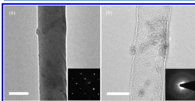
**Figure 2.** Melting process of an individual ZnTe nanowire during in situ heating and monitored by TEM. (a) The ZnTe nanowire at room temperature. Inset: the correspondent SAD pattern shows the crystalline structure of the nanowire. (b) The molten nanowire at 445 °C. The remaining oxide shell can be clearly seen from the image. The inset shows the SAD pattern without crystalline reflections. All scale bars are 50 nm.
