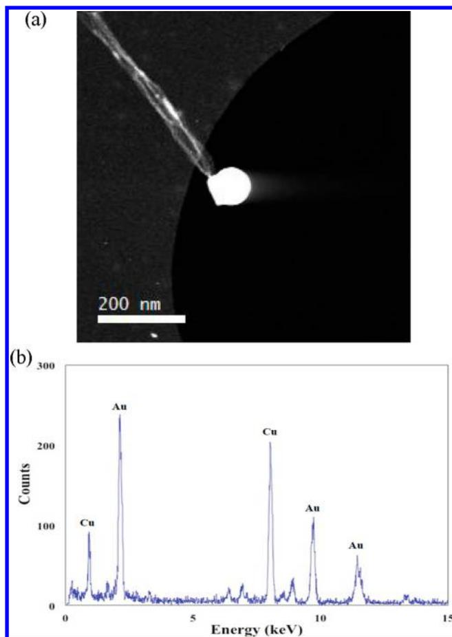
**Figure 5.** HAADF-STEM image of the molten ZnTe nanowire. The white part on the tip of the nanowire is an Au catalyst [confirmed by the EDAX analysis shown in (b)].
