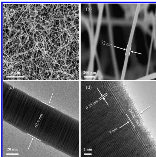
**Figure 1.** (a) SEM image of a mat of high-yield ZnTe nanowires grown by VLS technique. (b) Higher magnification SEM image of an individual ZnTe nanowire. (c) Low-magnification TEM image of a single ZnTe nanowire. (d) High-resolution TEM image of a ZnTe nanowire, showing a 3 nm oxide shell around the nanowire.
