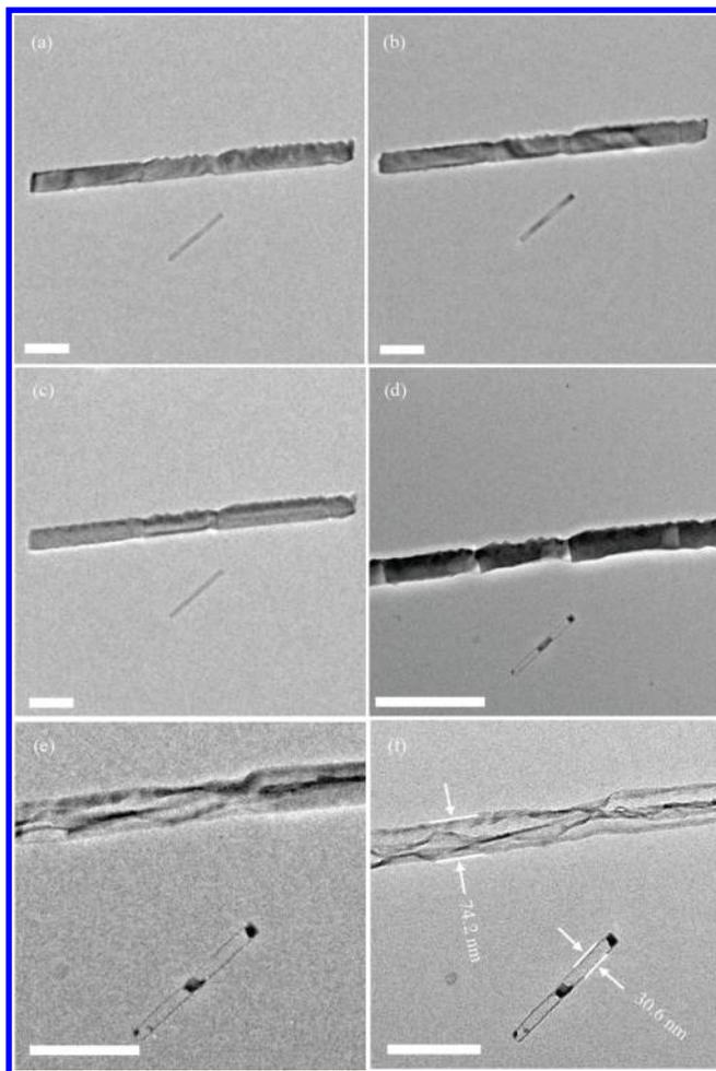
**Figure 3.** Low-magnification TEM images of two ZnTe nanowires (diameters of 31 and 74 nm) taken in a wide range of temperatures to study their melting behavior. (a–e) Different steps of the melting process at room temperature, 160, 320, 425, and 450 °C, respectively. (f) The final step of the melting process of the molten nanowires with a diameter of 31 and 74 nm. All scale bars are 200 nm.
