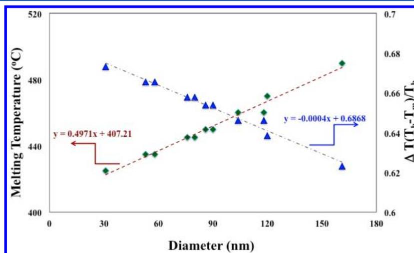
**Figure 6.** Measured melting temperature and the melting point suppression of ZnTe nanowires as a function of nanowire diameter.
