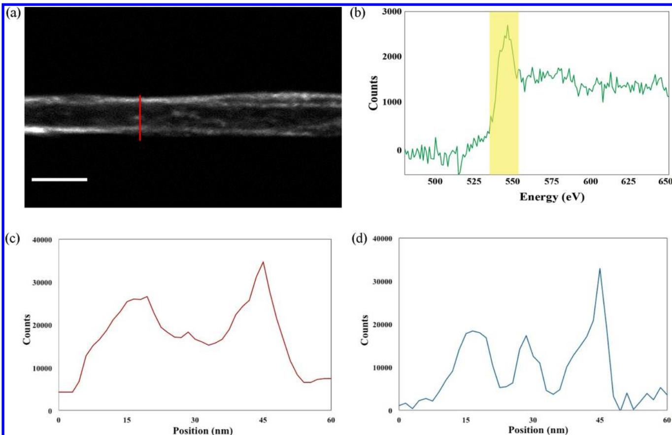
**Figure 4.** (a) A high-angle annular dark field (HAADF)-STEM image of a ZnTe nanowire after melting. The scale bar is 50 nm. (b) Measured EELS O K-edge at the shell around the ZnTe nanowire. (c) The brightness profile of the HAADF-STEM image along the red line shown in (a). (d) EELS line scan along the red line across the ZnTe nanowire shown in (a).
