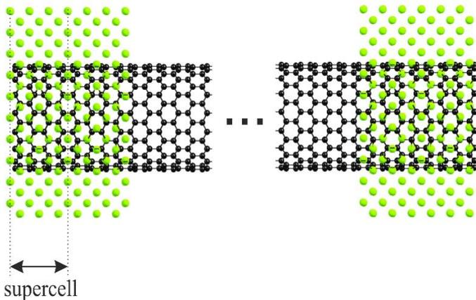
Fig. 1. Longitudinal view of the CNT-FET channel, embedded into the Pd
