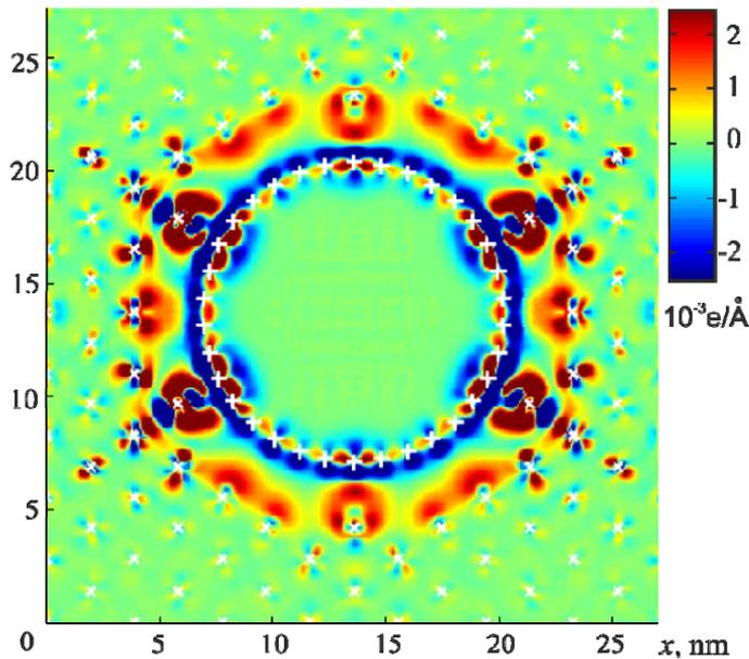
Fig. 4. Average surface charge density in the embedded nanotube (transverse direction). Positions of the Pd and C atoms is denote by symbols "x" and "+", respectively
