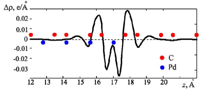
Fig. 5. Charge density difference near the external contact (averaged over transverse direction)
