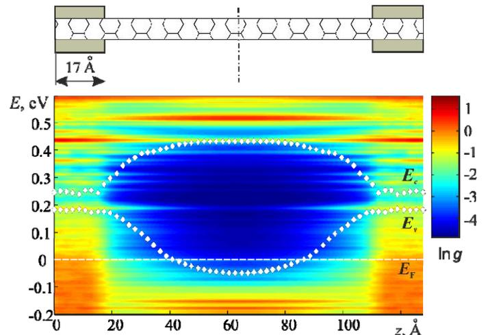
Fig. 2. Projected density of states  $g(E)$  onto carbon atoms along nanotube
