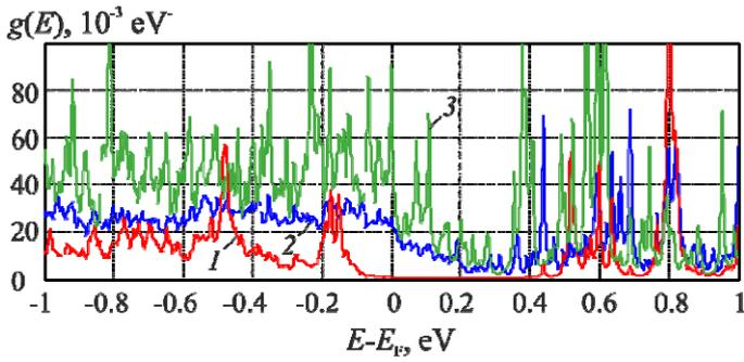
Fig. 3. Local density of states of the unit cell of CNT: at the center of the System 2 (1) ; at the embedded part of the CNT in System 2 (2); in the System 1 (3)
