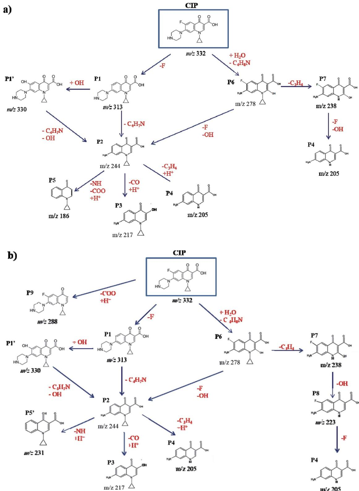
Fig. 3 Degradation mechanism of CIP photocatalytic degradation after 45 minutes of process with: (a)  $\text{TiO}_2$  and (b)  $\text{ZnO}$  nanoparticles. P1–P9 match the products assigned to the corresponding molecular ions.
