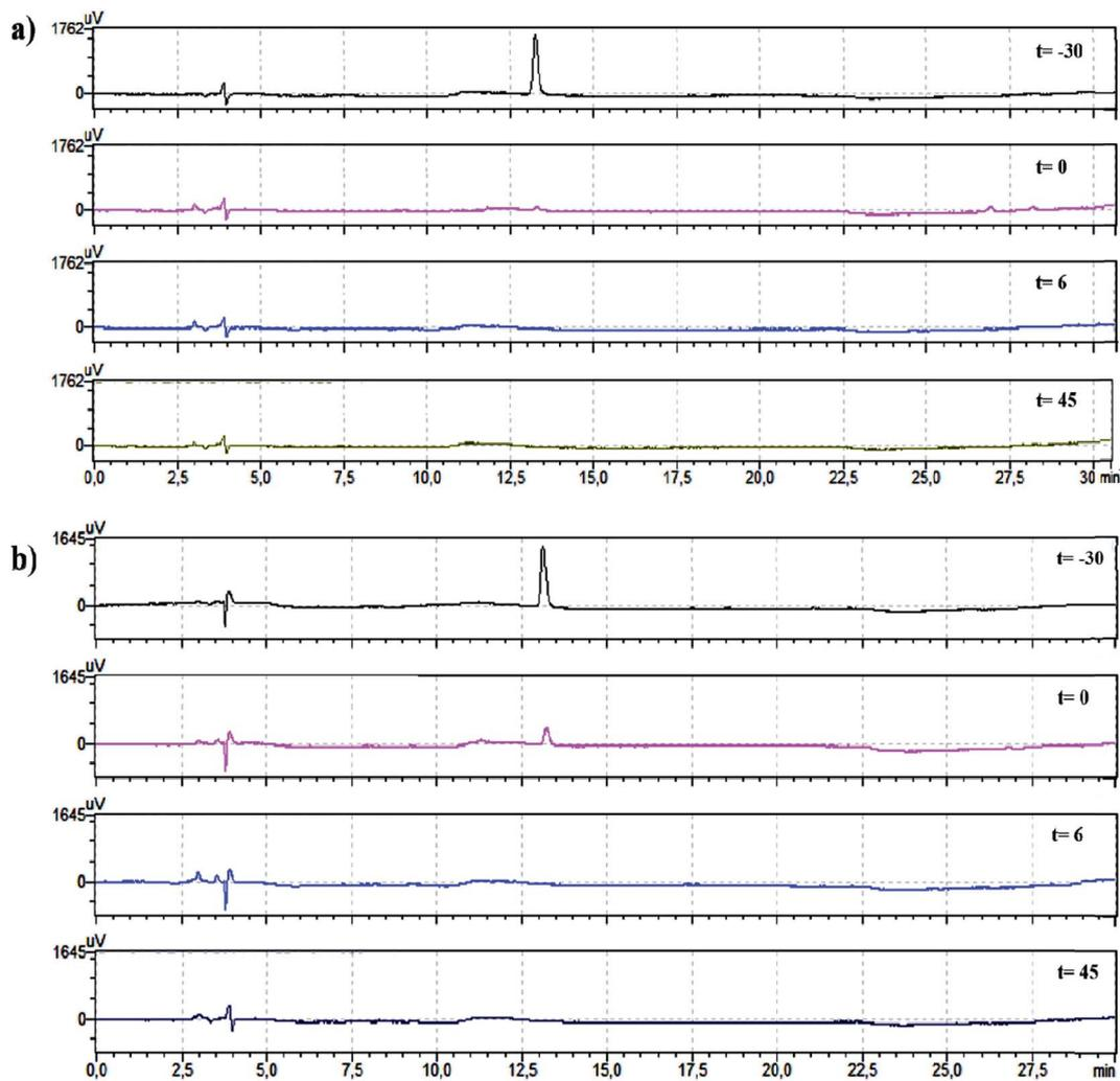
Fig. 1 HPLC analysis of CIP degraded samples with ZnO nanoparticles (a) and TiO<sub>2</sub> nanoparticles (b) at degradation times –30, 0, 6 and 45 min.
