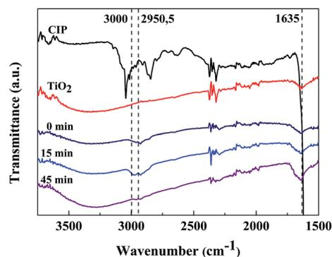
Fig. 2 FTIR analysis of CIP, TiO<sub>2</sub> nanoparticles and recovered TiO<sub>2</sub> nanoparticles after CIP photocatalytic degradation times 0, 15 and 30 minutes.
