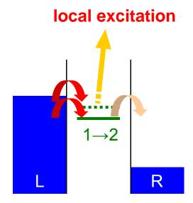
inelastic tunneling (vibration, spin flip) characteristic for molecules
