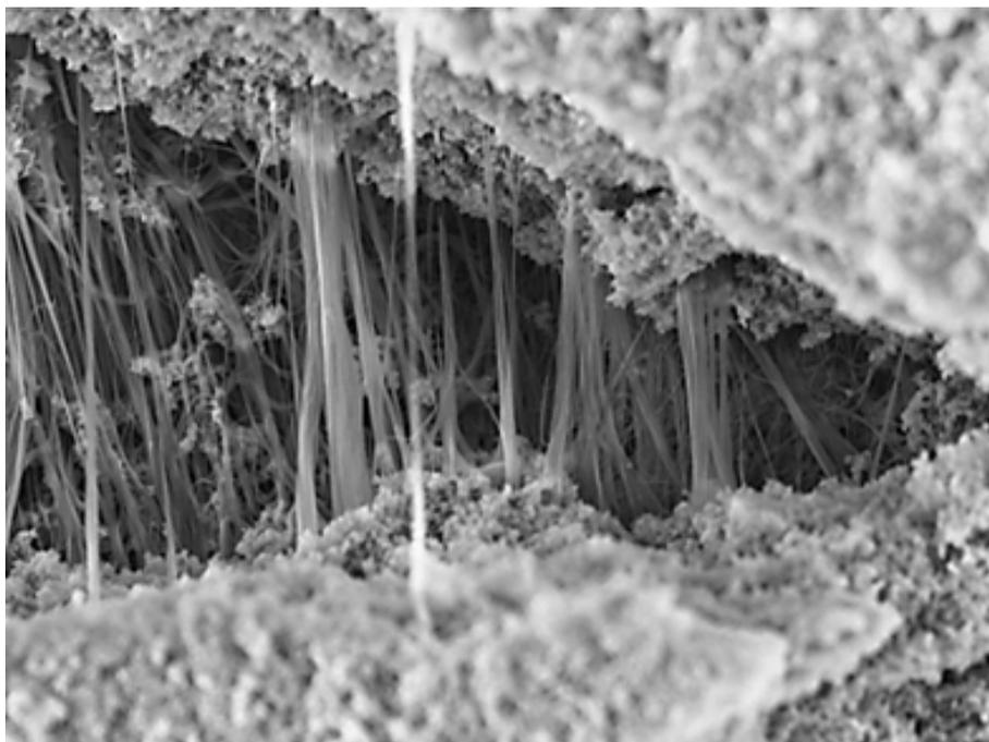
*Figure 2: A CNT forest in the alkali activated nanocomposite*
